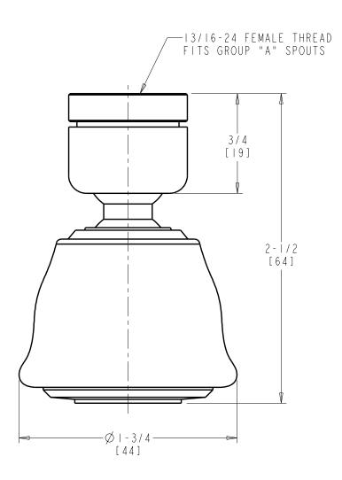
DIMENSIONS ARE IN INCHES AND [MILLIMETERS].
